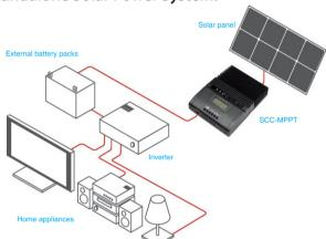
Combined MPPT technology and DSP controller, SCC-MPPT will convert best voltage to charge battery based on varied temperature. Compared to traditional solar charge controller, it allows your solar panels to operate at their optimum power output voltage, providing higher efficiency up to 97.8% with lower power loss.
