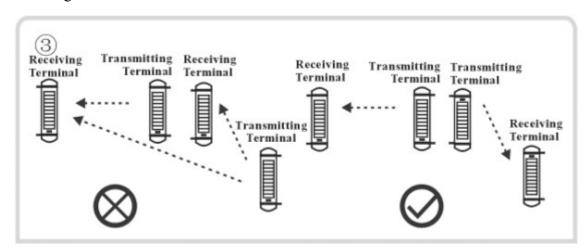
Note 3: Multiple light walls shall be installed for long-distance alarm in accordance with the installation instructions shown in the above-mentioned figure to avoid mutual interference among beams.
