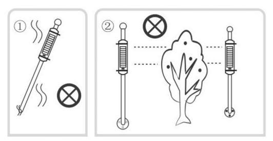
Note 1: Never inst all light walls at an inclined angle.
