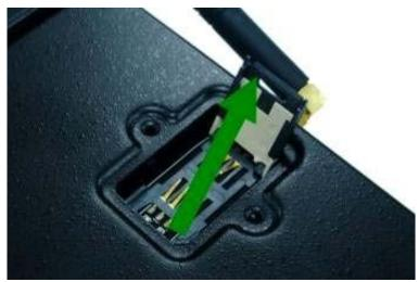
4). Insert the SIM card by sliding it into the card holder slot, with the chip module facing to the connectors on PCB, as shown in the picture.
