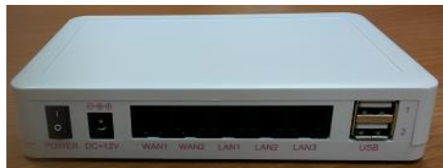
Rear view of SHS 3830
