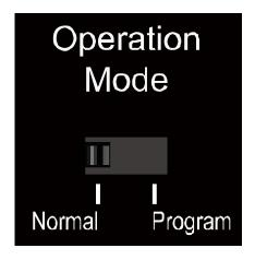
2. According to the silk prints nearby ("Program" for firmware update, "Normal" for RS232 transmission), change the switcher positions to set RS232 port's function.
