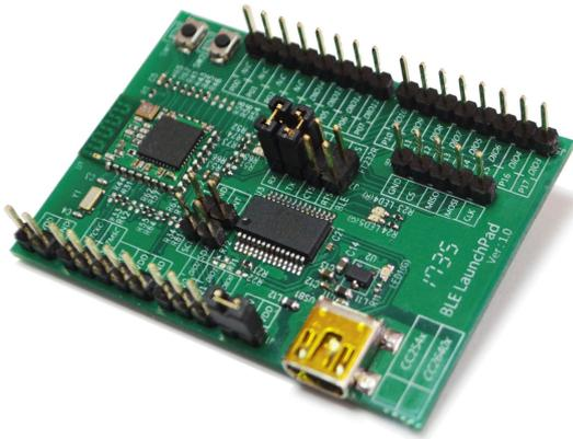
EVK-CC2541, BLE LaunchPad/ Development Kit, is an entire development kit for user to design Bluetooth Low Energy (BLE) application. It contains a Digimore Bluetooth module BT01-2 using TI Bluetooth low energy controller CC2541. TI CC2541 is a world-leading chip in Bluetooth Low Energy 4.0 and offers variety of peripherals such as UART, SPI, I2C and Timer.
