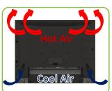
**Die-casting Housing**Patented fan-less design with ventilation holes allows heat to escape. (For Core i3, i5 & i7 only)
