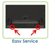
Just two screws to reach the major components, such as MB, LCD,...etc.
