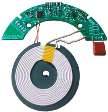
The WCM-TP6735 is a Wireless Power digital controller for Qi Compliant Wireless fast charger. The design of this module is based on the WPC Qi 1.2 standard. The module uses a dedicated wireless charging chip and an efficient & highly integrated driving full-bridge chip. The charging efficiency can reach 81%. The WPC standard V1.2 has input over-voltage, over-current, output over-voltage, over-current, and over-temperature protection functions. LED lights indicate the module's working status.
