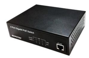
switch complies with IEEE 802.3af and 802.3at standards and supplies up to 30W per port, with a total PoE power budget of 65W or 120W. It automatically detects IEEE 802.3af/at compliant device connected and provides power and data over a RJ45 cable to these devices.
